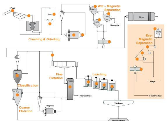
Similar to the equipment used in wet processes, Eriez uses drum, roll, pulley and filter type magnetic separators in varying degrees of intensity to process dry minerals. These processes require conveyors, feeders and belts to present the material to the magnetic separators in underbelt, overbelt or gravity-fed applications.
